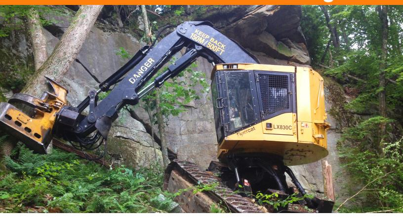
The 5185 is a robust fixed wrist bar saw for wheel or track carriers. With powerful cutting and grapple arm performance, the 5185 is ideal for felling, limbing, topping and shoveling large, high value timber.
