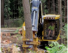
High torque 340° wrist for increased versatility and reduced machine travel.
