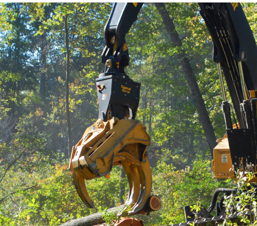
High capacity rotator with clean hose routing and continuous rotation.
