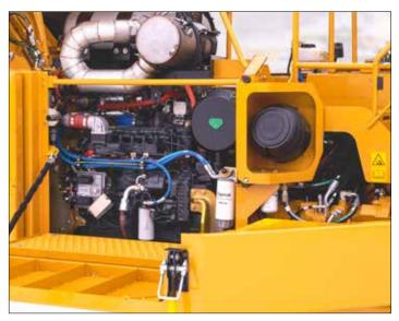
The engine and hydraulic pumps are compartmentalized and easily accessed. Easy access to daily service points.
