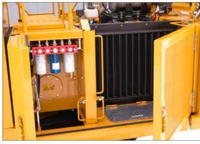
Swing-out doors access filters and cooling system components for quick daily service.
