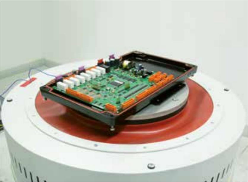
Electronic and hydraulic components on the truck-mounted crane are subjected to extremely high environmental loads. In the environment simulation lab, all electronic and hydraulic components are subjected to the respective test procedures.
