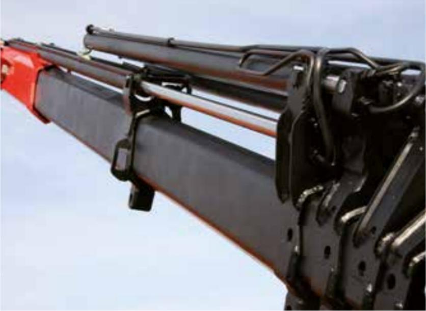
PALFINGER cranes are designed in every detail for ease of servicing and maintenance. For example the low maintenance extension boom system significantly reduces the usual maintenance expenditure. No further servicing work is required after one-off initial lubrication using a special food grade grease.
