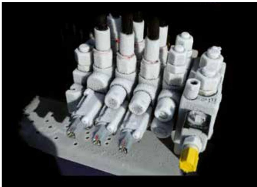
We test the most important components (control spool and electronic components) in the climate exposure test cabinet, which simulates tough, real conditions (extremely low and/or high temperatures, temperature fluctuations, air humidity,...).
