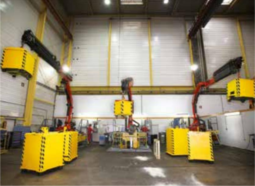
PALFINGER cranes are assembled in team manufacturing. And, before they leave the plant, they have passed a lot of tests. The highest quality standards require strict and meticulously accurate testing methods. Therefore, at PALFINGER, every crane passes through an extensive check on the test bench. With the help of special test software, successive execution of the stipulated testing steps takes place on the basis of specifically defined master test plans.
