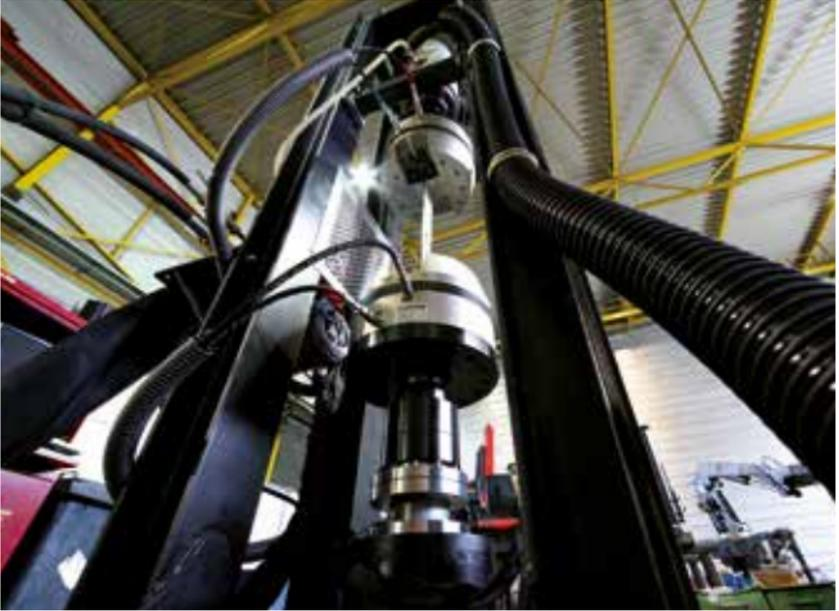
By using expansion measurements and automatic endurance tests, PALFINGER cranes are tested for the expected service life even before the start of production and within a few months. The components are subjected to the harshest loads on modern hydropulser test benches to be able to offer top quality products. With this technology, it is possible for PALFINGER to optimize components to meet the harshest customer demands.
