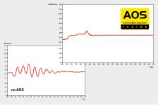
The active oscillation suppression system prevents "post-oscillation" in the event of rapid braking or load changes. The stress peaks on the extension boom system are reduced and material fatigue and wear are minimized. This increases the resale value.
