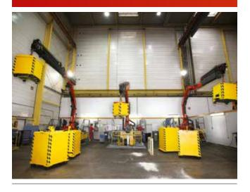
PALFINGER cranes are assembled in team manufacturing. And, before they leave the plant, they have passed a lot of tests. The highest quality standards require strict and meticulously accurate testing methods. Therefore, at PALFINGER, every crane passes through an extensive check on the test bench. With the help of special test software, successive execution of the stipulated testing steps takes place on the basis of specifically defined master test plans.
