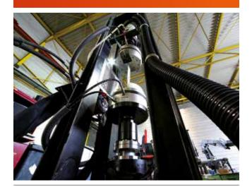
By using expansion measurements and automatic endurance tests, PALFINGER cranes are tested for the expected service life even before the start of production and within a few months. The components are subjected to the harshest loads on modern hydropulser test benches to be able to offer top quality products. With this technology, it is possible for PALFINGER to optimize components to meet the harshest customer demands.
