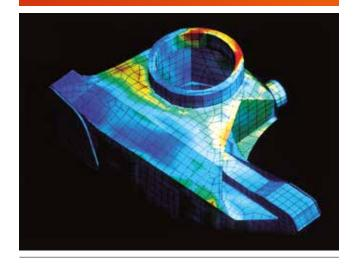
High-tech in crane design - all load-bearing components are calculated with finite element technology, which has been used for years. They are optimized and designed to be weight-saving. Years of development edge - PALFINGER's ideas are repeatedly copied and many of solutions developed by PALFINGER become the technical standard in crane construction over the years
