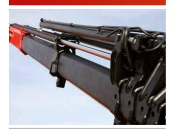
PALFINGER cranes are designed in every detail for ease of servicing and maintenance. For example the low maintenance extension boom system significantly reduces the usual maintenance expenditure. No further servicing work is required after one-off initial lubrication using a special food grade grease.
