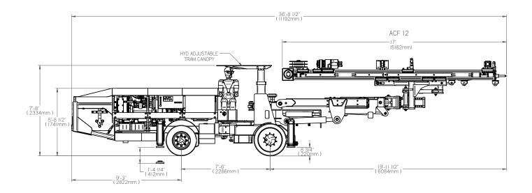
Fletcher model J101-AD/E is a diesel tram, electric drill jumbo for narrow vein mining applications in headings up to 22m<sup>2</sup>. The rig is nimble in tight quarters with proportional control on tram and boom functions. Drilling efficiency is optimized with direct acting anti-jam circuit and a variety of rockdrills for various rock conditions.
