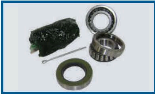
WHEEL BEARING TRAILER KITS SERIES TK0750, TK1000, TK1063, T K1125, TK3500
